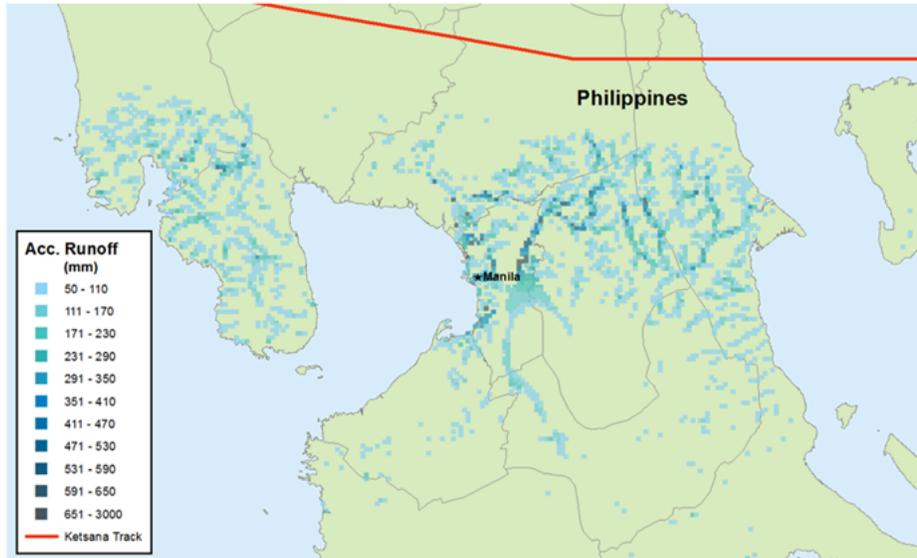
**Figure 98. Storm track and modeled accumulated runoff for Typhoon Ketsana (2009)**
