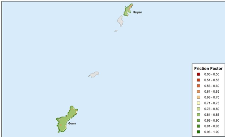
**Figure 87. Verisk friction factors used in the Verisk Typhoon Model for the Northwest Pacific Basin – Guam and Saipan**
